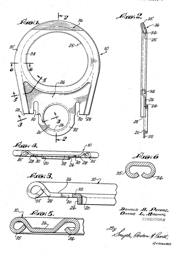
RING-SHAPED TAB FOR TEAR STRIPS OF CONTAINERS
